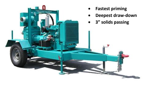
CDPW's unique oil bath system provides constant lubrication to the bearings and mechanical seal allowing the ability to be used in conditions with intermittent flows and suction lifts to 25 feet. Pumps are designed to pass up to 3" solids commonly found in construction dewatering, pond drainage or municipal wastewater. CDPW pumps are known for being robust in a variety of conditions.
